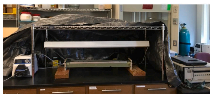
b) Reaction chamber for plate samples
