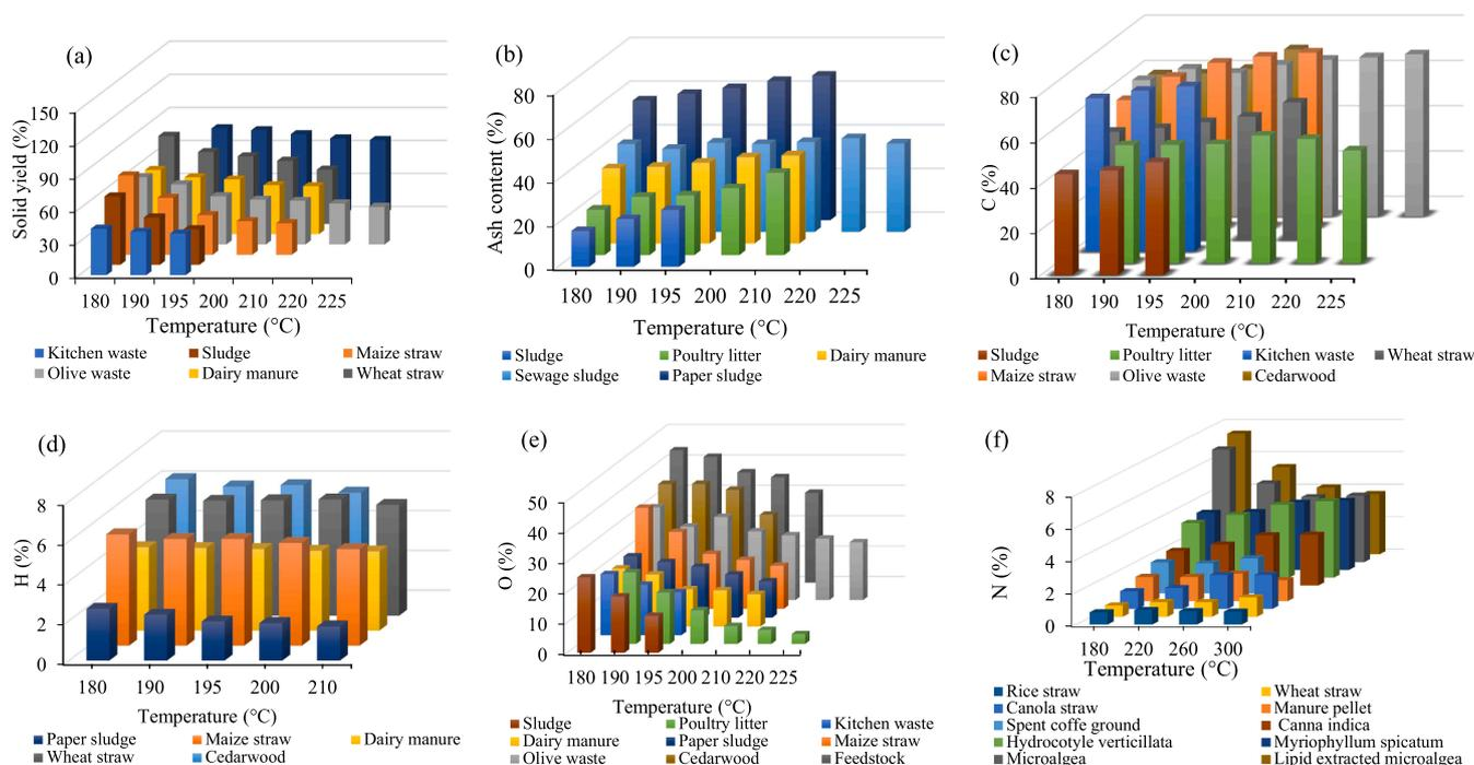
**Fig. 2.** Effect of heating temperature on (a) hydrochar yield, (b) ash content, (c) C content, (d) H content, (e) O content, and (f) N content. Generally, the changes in hydrochar characteristics depend on the type of feedstock and HTC conditions. Data obtained from the reported studies [14,33,47,85,88–101]
